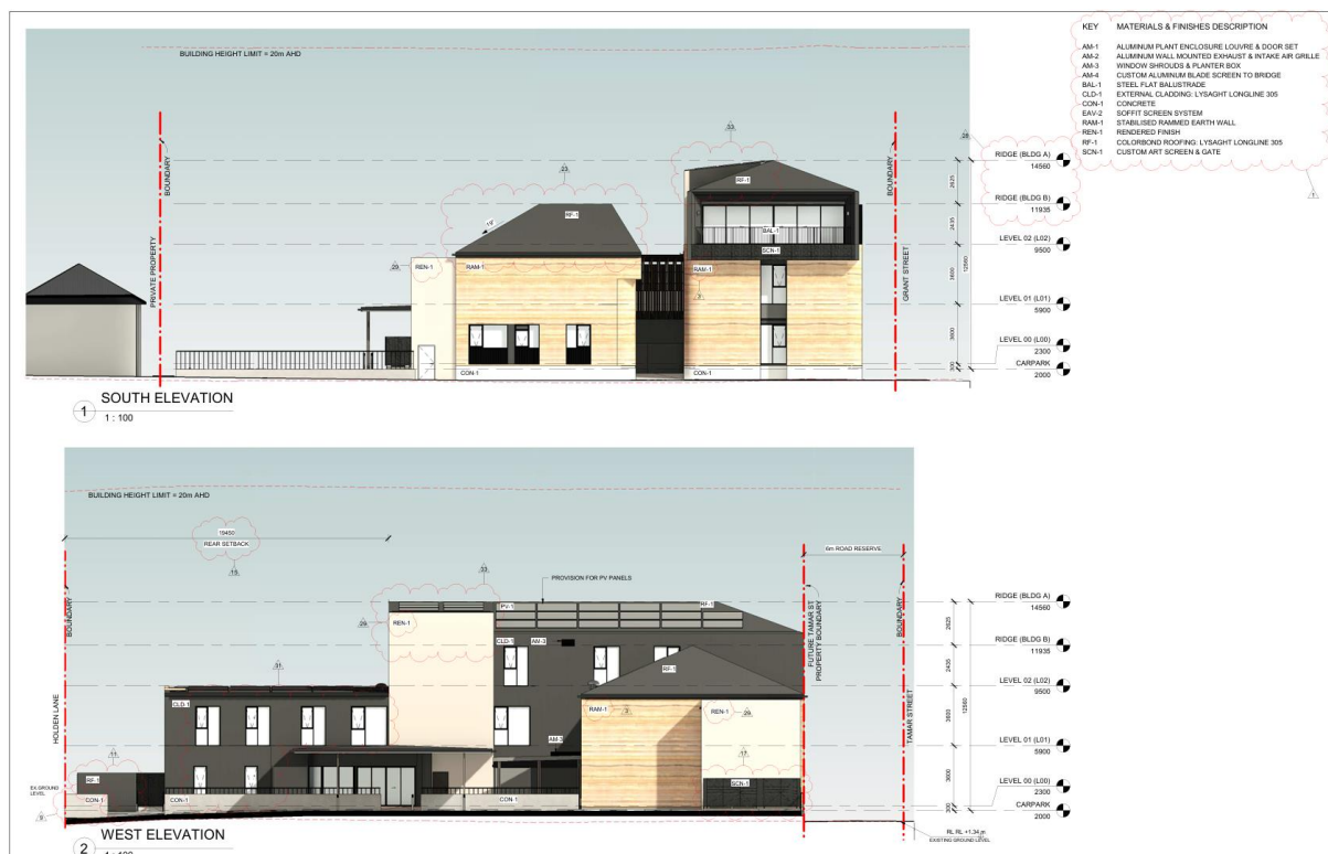
Figure 7- South and West Elevation. Source: Kaunitz Yeung Architecture
